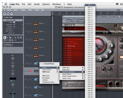
Figure 5-9: Assigning a Logic Pro MIDI track to the MOTU Symphonic Instrument audio instrument, which in this example is Audio Instrument 1.
