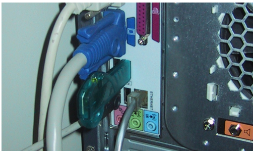
Figure 2-1: The MOTU Symphonic Instrument requires the USB iLok SmartKey (included).
