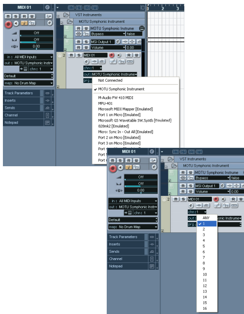
Figure 5-20: Assigning a MIDI track to the MOTU Symphonic Instrument and choosing a MIDI channel.
