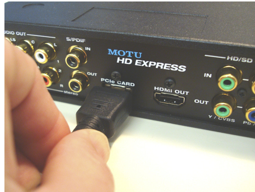
Figure 4-4: Making the connection from the computer to the HD Express.
