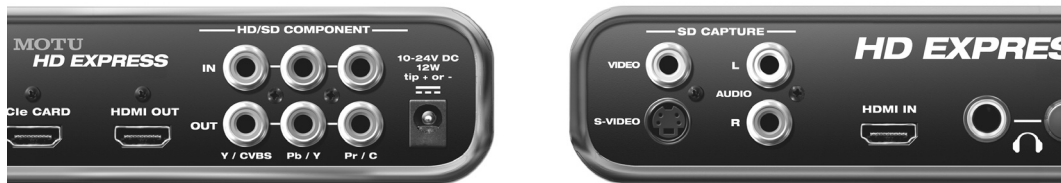
Figure 4-5: The HD Express video connectors.
