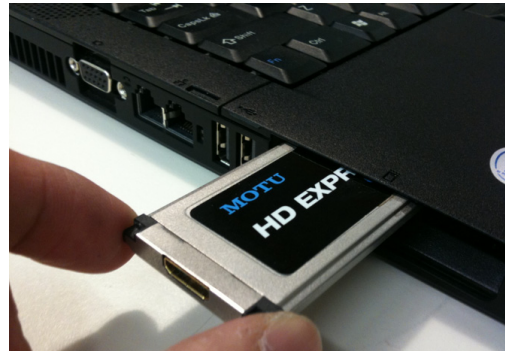
Figure 4-2: Inserting the HD Express ExpressCard adapter.
